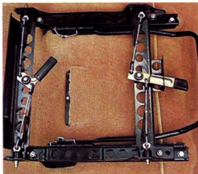
Volvo's front seat frame, securely anchored at four points.
