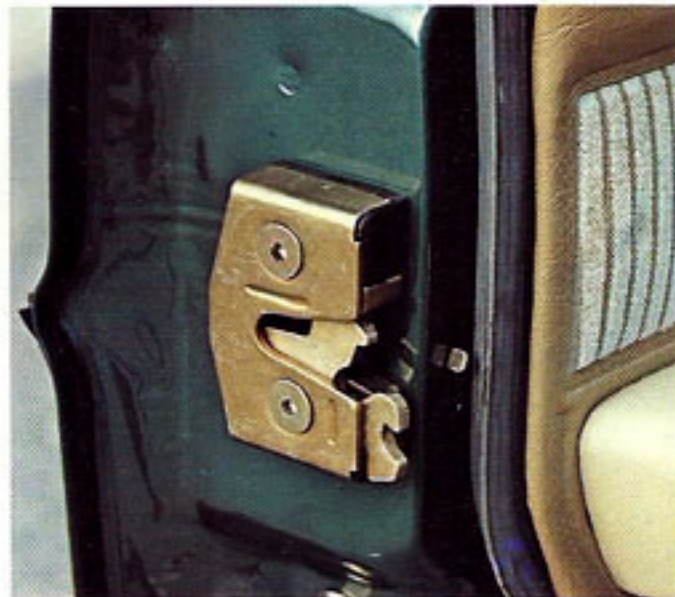
Door latches have built-in drains; water that gets in runs out.
