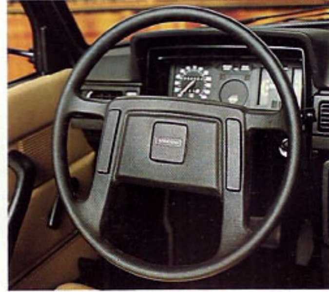
Padded safety steering wheel, variable-intensity illuminated instrumentation.
